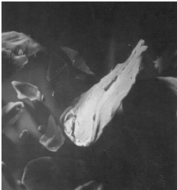
Fig. 8. SEM scan at 25 kV of the pectin extracted by traditional heating method, X150, original width of picture was 200 μm. This figure and Fig. 7 are under the same conditions, but they describe the difference from the different angle and side.
